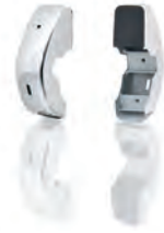
Bumper guard Part no. 90150503151 (left) 90150503251 (right) For S trim (with plastic cover), with holes for rubber buffer. 911 F model (1969–1973)
