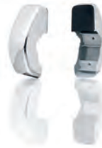
Bumper guard Part no. 90150503126 (left) 90150503226 (right) For standard trim (with plastic cover), without holes for rubber buffer. 911 F model (1969–1973)
