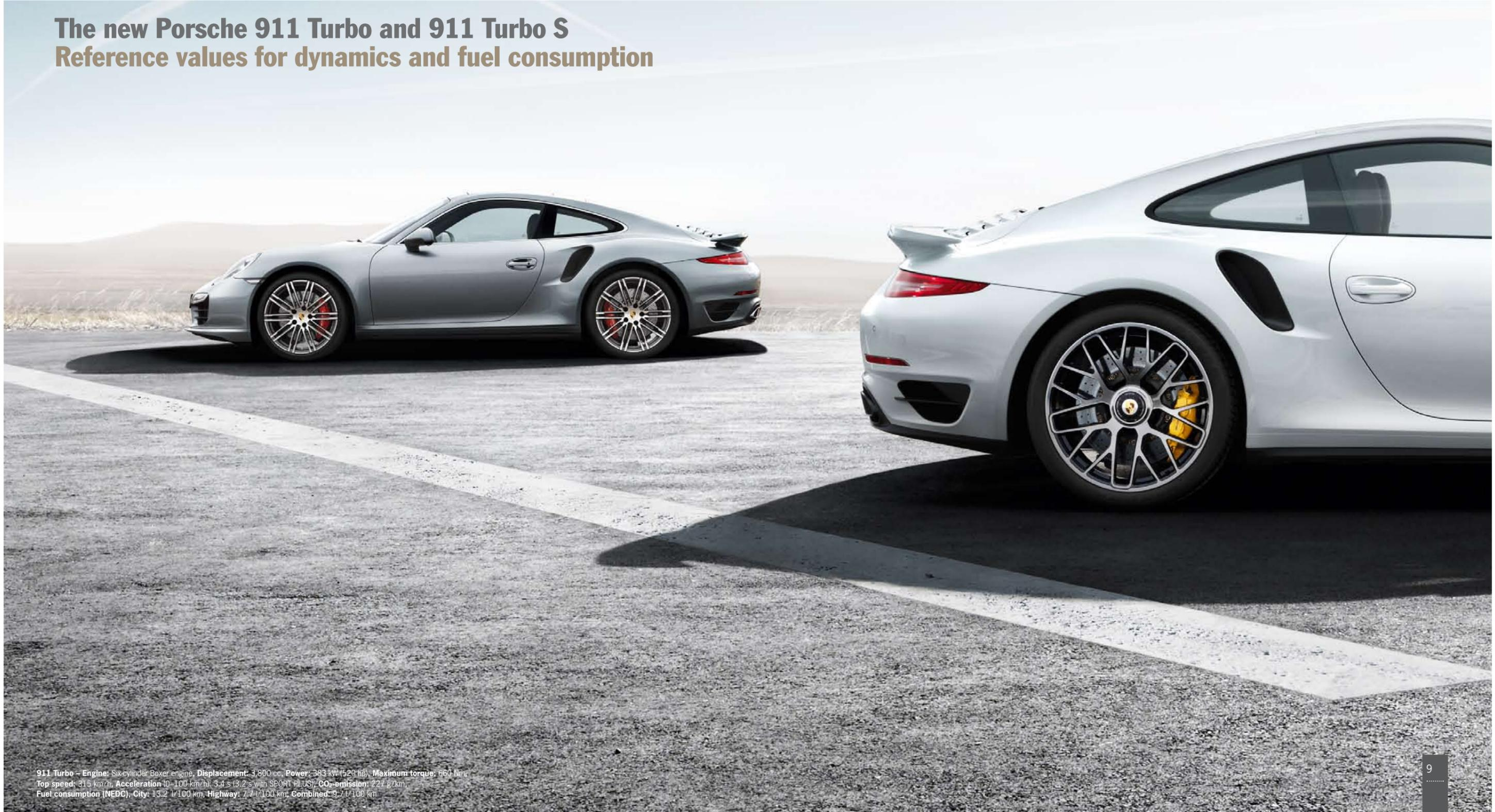
**911 Turbo** – Engine: Six-cylinder Boxer engine, Displacement: 3,800 cc, Power: 383 kW (520 hp), Maximum torque: 660 Nm, Top speed: 315 km/h, Acceleration (0–100 km/h): 3.4 s (3.2 s with SPORT PLUS), CO<sub>2</sub> emission: 227 g/km, Fuel consumption (NEDC), City: 13.2 l/100 km, Highway: 7.7 l/100 km, Combined: 9.7 l/100 km
