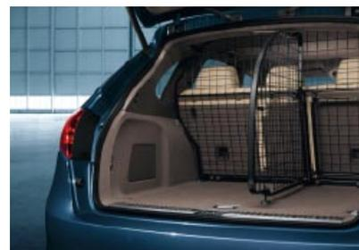
**Dividing grid including luggage compartment Divider:** an effective steel restraint system with a grid covering the entire area behind the rear seats to protect passengers. With luggage compartment overflow into sitting area for skis and long loads.
