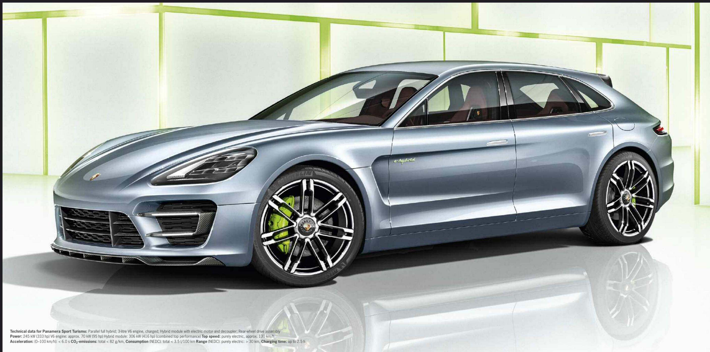
**Technical data for Panamera Sport Turismo:** Parallel full hybrid; 3-litre V6 engine, charged; Hybrid module with electric motor and decoupler; Rear-wheel drive assembly
