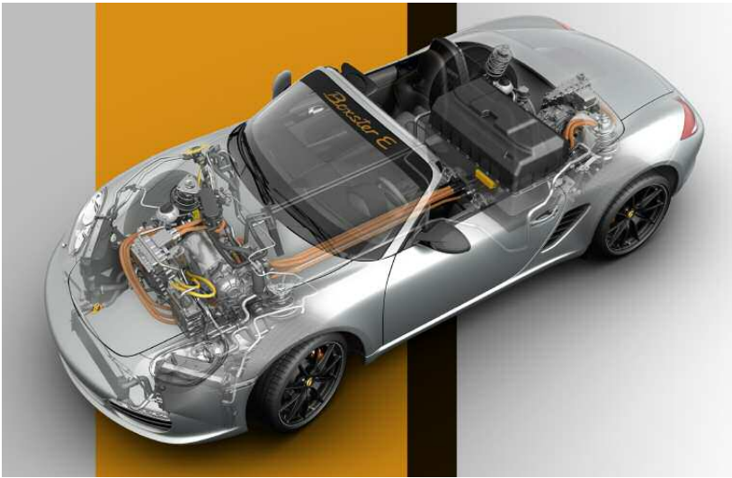
E as in Efficient: Two electric motors working independently from each other drive the front and rear axle
