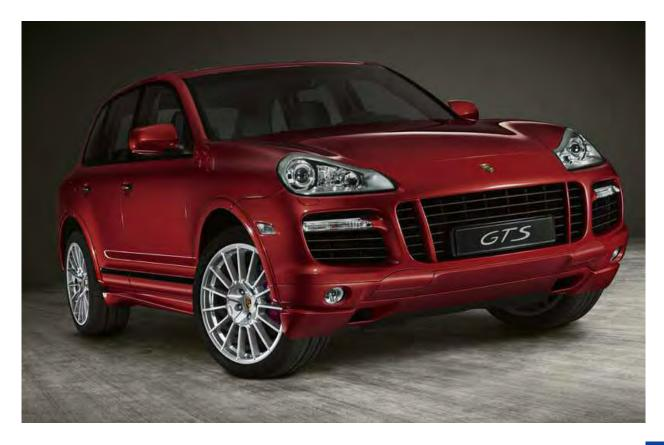
are the same as those of the Cayenne Turbo, and the striking 14 mm wheel arch widenings offer plenty of room for the standard 21-inch alloy wheel rims with 295/35 R21 tyres. In addition, two new colours have been developed exclusively for the GTS: GTS Red and Nordic Metallic Gold.
