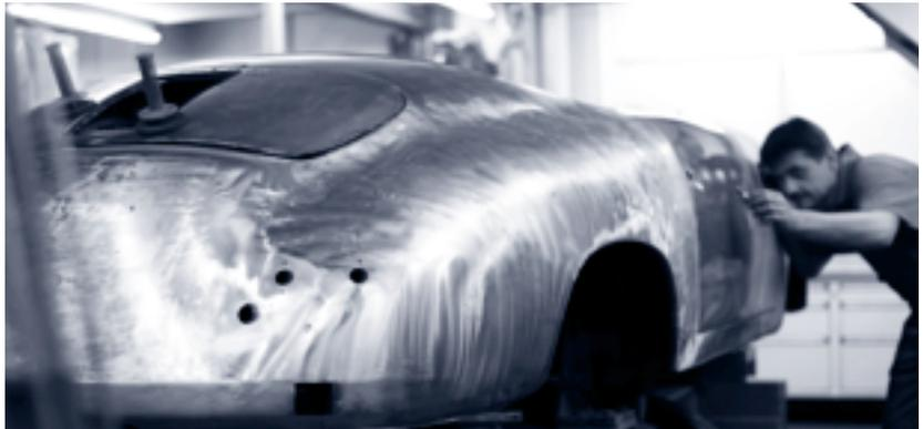
workshop, from the spoiler right up to the complete GRP body. We have repaired wings and nose and tail sections of the 959, panelling in the Porsche 917 and many other parts of particularly exclusive vehicles from the Porsche product range.
