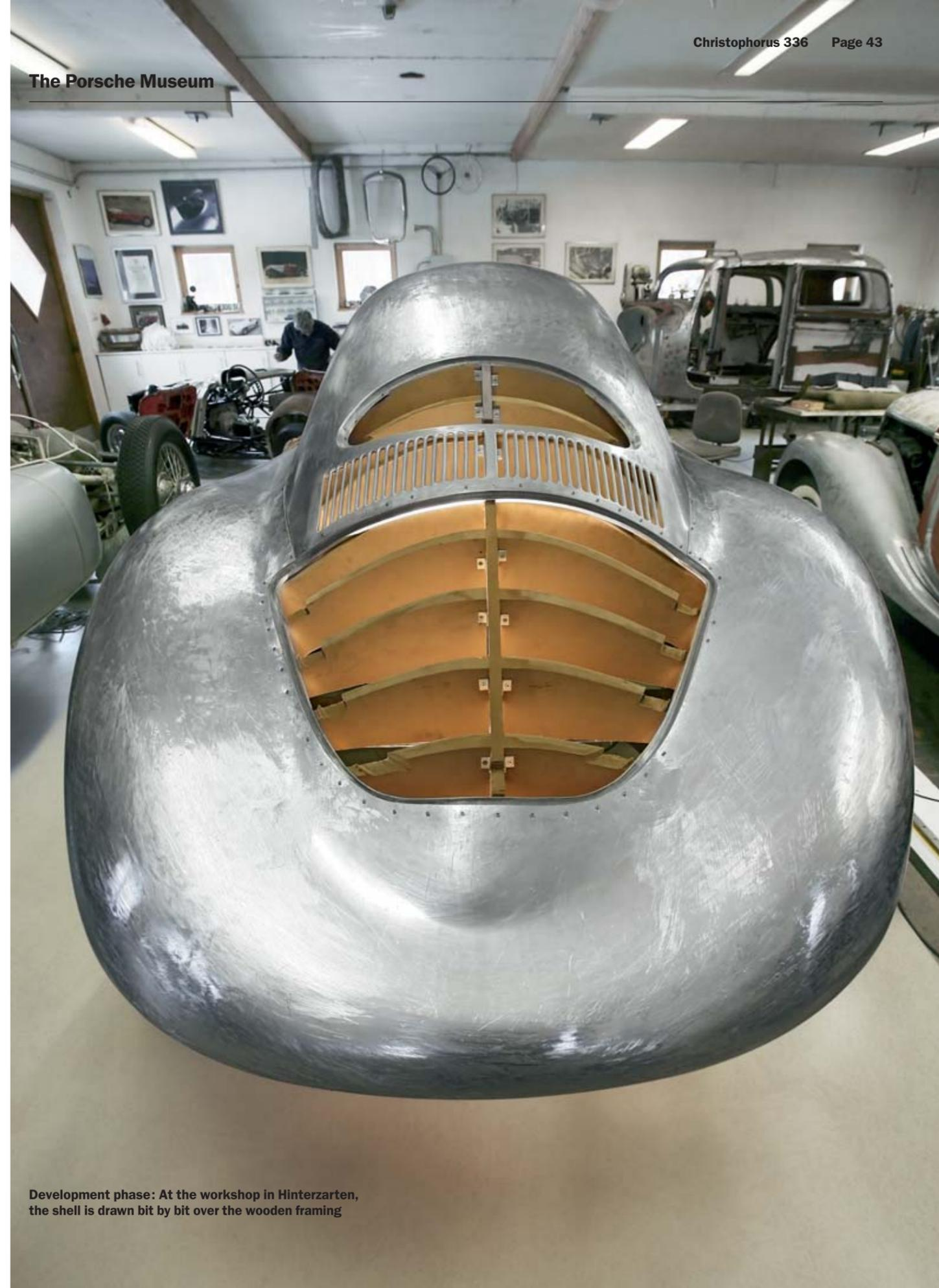
**Development phase:** At the workshop in Hinterzarten, the shell is drawn bit by bit over the wooden framing
