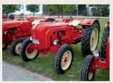
**Engine:** Three-cylinder with 2,467 to 2,625 cc **Power output:** 30 to 40 bhp at 2,000 to 2,300 rpm **Curb weight:** 1,985 to 2,450 kg (4,376–5,401 lbs.) **Curb weight:** 1,788 to 2,450 kg (3,941–5,401 lbs.)
