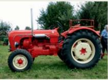
**Engine:** Four-cylinder with 3,288 to 3,500 cc Power output: 50 bhp at 2,000 rpm
