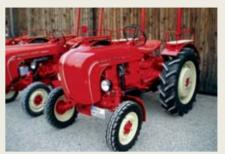
**Power output:** 20 to 30 bhp at 1.950 to 2.300 rpm **Curb weight:** 1,110 to 1,510 kg (2,447–3,330 lbs.) **Speed:** 19 to 20 km/h
