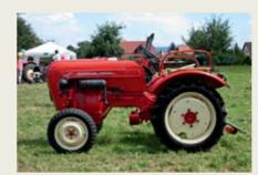
Engine: One cylinder with 822 to 875 cc. **Power output:** 12 to 15 bhp at 2,200 to 2,250 rpm **Curb weight:** 845 to 1,000 kg (1,863–2,204 lbs.) **Speed:** 16.5 to 20 km/h
