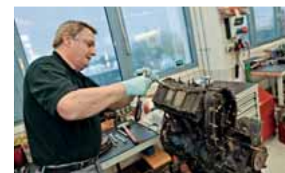
Not just the right spin: The six-cylinder boxer engine with 2.4-liter displacement was completely taken apart
