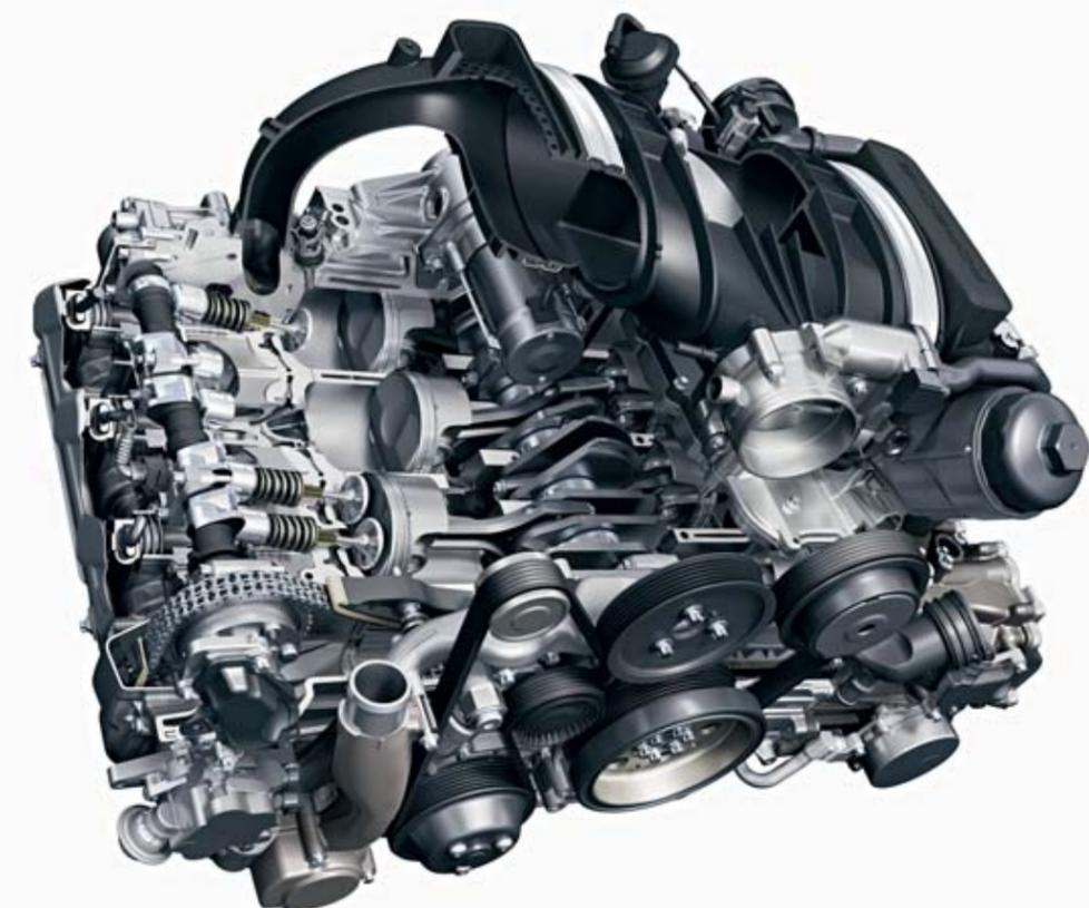
**Engine of the Year: The 3.8-liter engine is mightier than its predecessor—yet in conjunction with PDK, fuel consumption is reduced by about 13 percent, and CO<sub>2</sub> emissions by nearly 15 percent**
