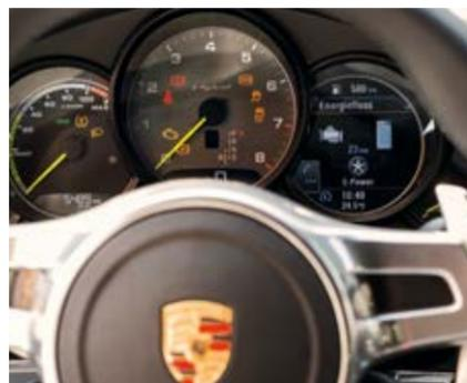
Of the three main gauges, the one on the right shows energy flow and range
