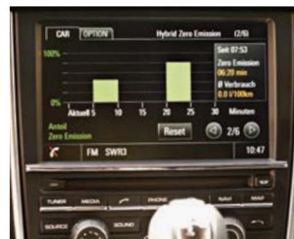
No fuel consumption: The hybrid display shows zero-emission driving
