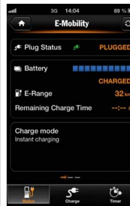
Porsche Car Connect is a further developed version of already existing online services from Porsche. This new car-oriented service is based on its own architecture, which connects the car to a server by means of an internal communications unit and the mobile phone network.
