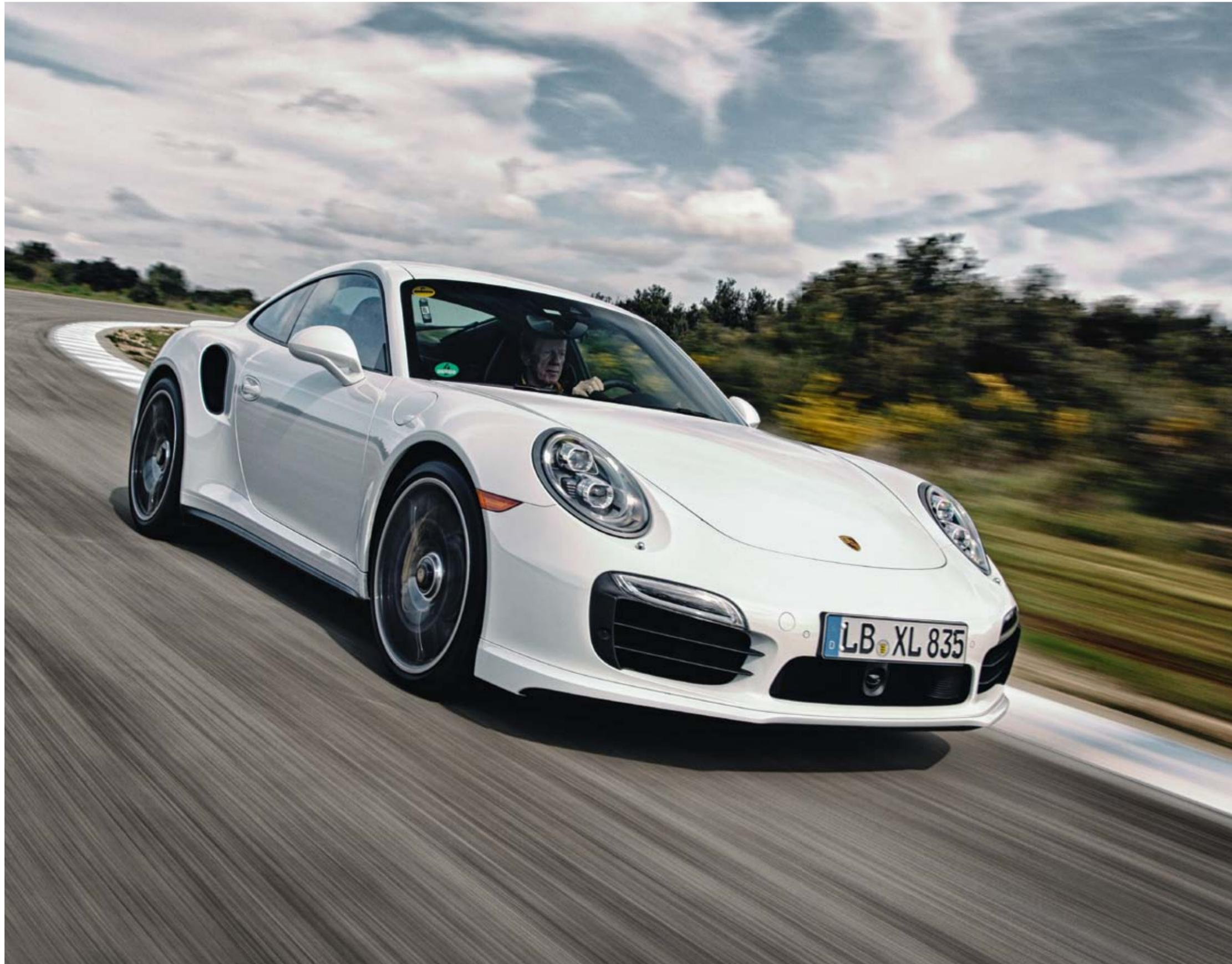
Standard LED main headlights distinguish the Turbo S from the Turbo, while the rear axle aids steering for the first time
