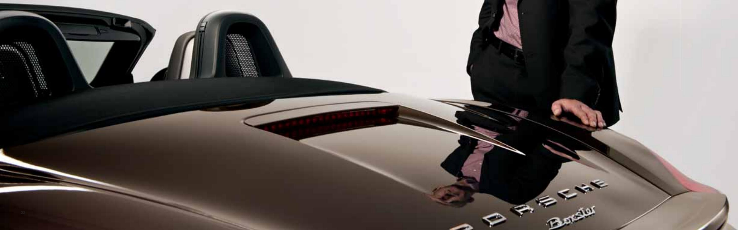
were able to realize dual air intakes.” Wöhler is happy to elaborate: “Before, the engine took air in on one side only, and on the other side it got cooling air. Now air comes in through both openings in front of the rear wheels. Having a lot of air means more power—and the voluminous sound it makes is great too.”
