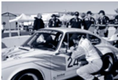
Would that put an end to racing? No. The very well prepared team not only had a spare engine on hand but a complete vehicle to act as a spare parts carrier. The input shaft was very quickly removed from the spare vehicle but the wheel hub had to be changed as well because the gearing on the spare part did not fit the new vehicle. Unbelievable though it may sound, the Porsche was on its way again within 20 minutes – in place 39.
