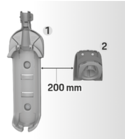
Fig. 7: Distance from wall mount to plug holder
