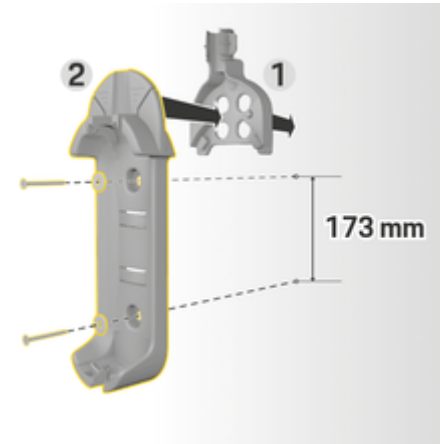
Fig. 3: Drilling dimensions
