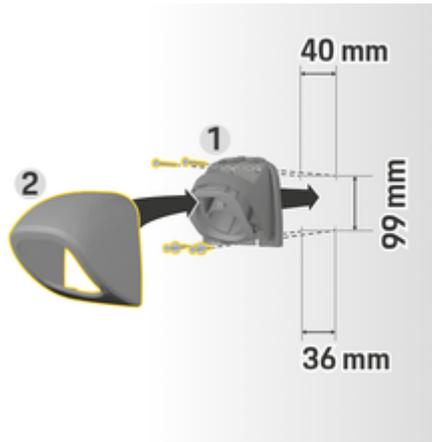
Fig. 8: Drilling dimensions
