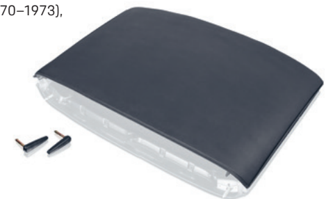
Complete Targa roof, embossed outer cover Part no. 91156500240 911 G model (1974–1984), only for Targa
