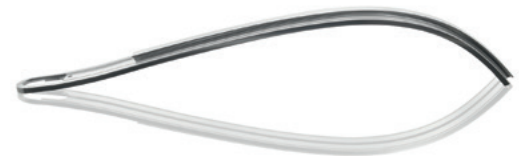
Trim strip Part no. 91150509700 911 F model (1972–1973), only for Carrera RS 2.7
