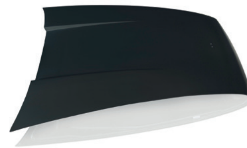
Bonnet made of thin sheet metal Part no. 90151101023GRV 911 F model (1972–1973), only for RS 2.7
