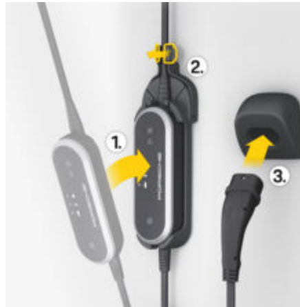
Fig. 11: Inserting control unit
