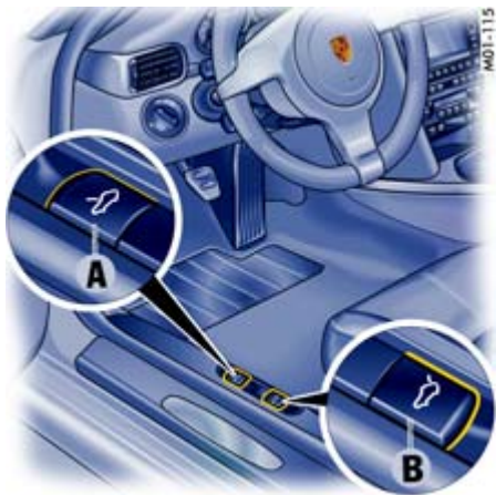
A - Opening the luggage compartment lid B - Opening the engine compartment lid
