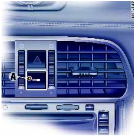
A - Light-emitting diode for alarm system
