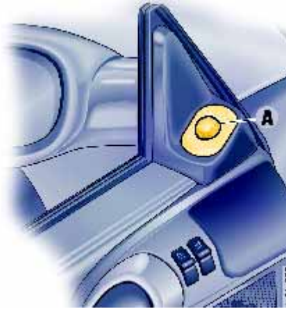
A - Control switch for door mirror adjustment
