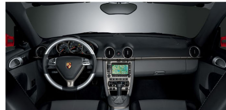
▲ Cayman dashboard with optional equipment, e.g., leather interior package with two-tone combination, PCM, 3-spoke multifunction steering wheel with AluLook trim.
