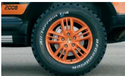
Off-road tyres by BF Goodrich increase ground clearance by 30 mm
