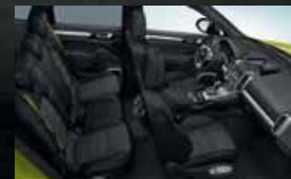
The GTS sports seats with 8-way adjustment are extremely sporty thanks to their low positioning. With adjustable fore/aft, height and squab/backrest angle settings, they also offer exceptional comfort and support – even during performance driving. All the door panels, armrests,
