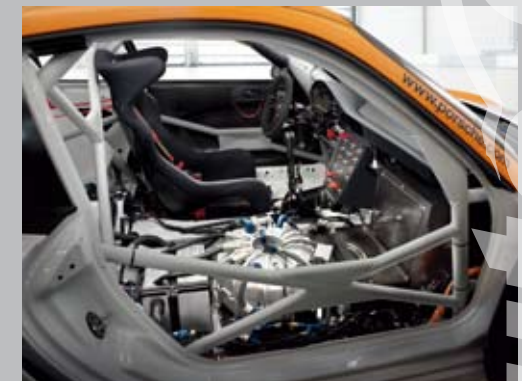
A revolutionary flywheel beside the driver collects kinetic energy then injects again for additional power and performance.
