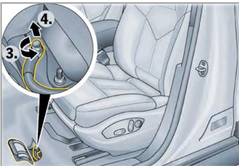
3. Disconnect the 12-volt battery's ground cable from the screw terminal (-3-).
