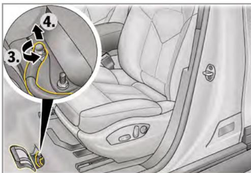
3. Detach the negative cable of the 12-volt battery at the threaded connection (-3-) and secure it against unintentional contact (-4-).
