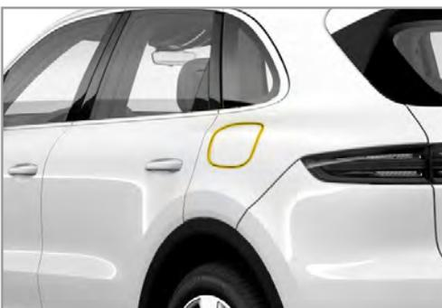
**Vehicle charging connection** behind the charging-socket lid on rear left side of the vehicle
